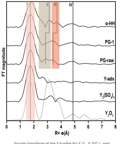
Fourier transform at the Y K-edge for  $Y_2O_3$ ,  $Y_2(SO_4)_3$  and Y-ads model compounds, and PG, PG-1 and  $\alpha$ -HH samples.
