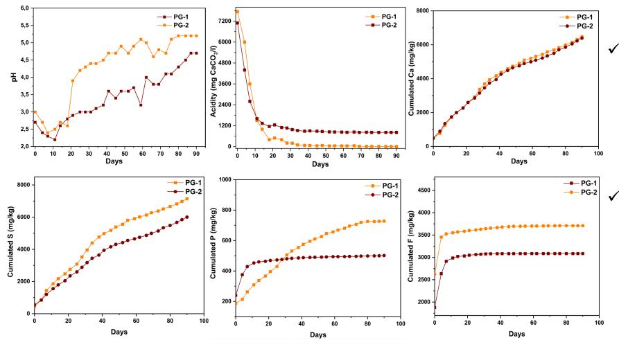
High acidity of the phosphogypsum samples in the first leaching days caused by the presence of intrinsic residual acid.
